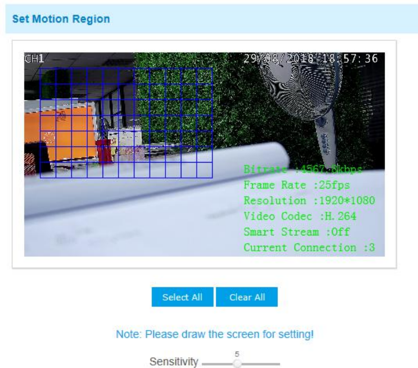
Figure 2 Motion Detection Settings on IP Cameras
