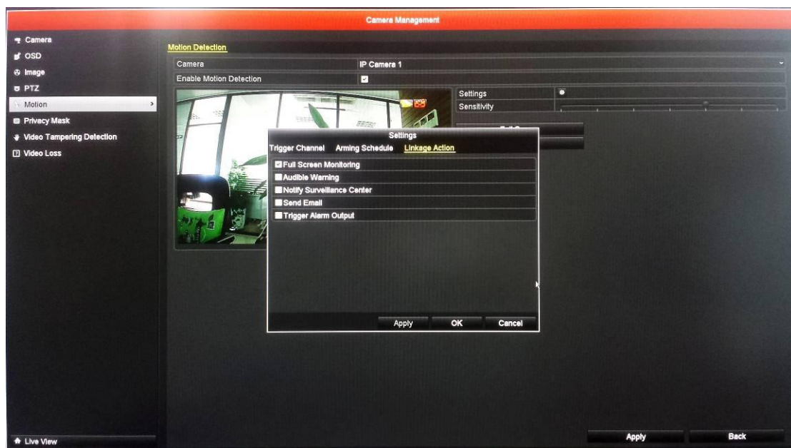
Figure 7 Motion Detection Settings on the NVR
