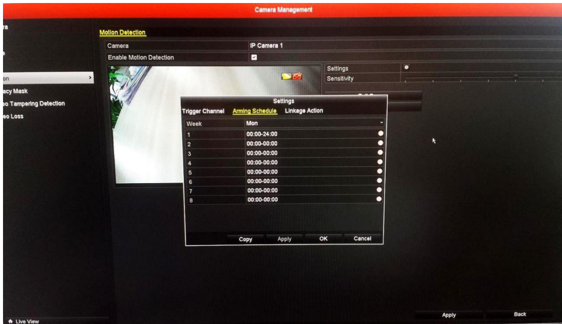
Figure 6 Motion Detection Settings on the NVR
